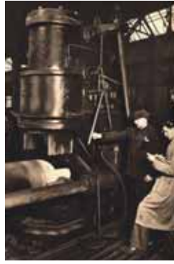
Forming of the tube end The fifties
