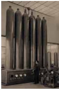
Accumulators for hydropneumatic plant 1940-1950
